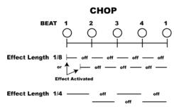
64, then smaller increments making for another interesting effect. When the effect is first activated the music will play the section then turn off for a section. This is important because you can reverse the sections that are off and on by activating the effect in the other section. If you deactivate the effect then turn it on again it remembers the last set parameter.
